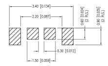
\*UNLESS OTHERWISE SPECIFIED TOLERANCES PER DECIMAL PRECISION ARE:  $x=\pm1$  (±0.039),  $x.x=\pm0.5$  (±0.020),  $x.xx=\pm0.25$  (±0.010),  $x.xxx=\pm0.127$  (±0.005). LEAD SIZE=±0.05 (±0.002), LEAD LENGTH=±0.75 (±0.030). MIN =  $\frac{+0.00}{-0.00}$  MAX.=  $\frac{+0.00}{-0.00}$
