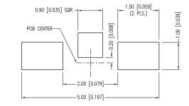
\*UNLESS OTHERWISE SPECIFIED TOLERANCES PER DECIMAL PRECISION ARE: X=±1 (±0.039), X.X=±0.5 (±0.020), X.XX=±0.25 (±0.010), X.XXX=±0.127 (±0.005). LEAD SIZE=±0.05 (±0.002), LEAD LENGTH=±0.75 (±0.030). MIN=  $\frac{+DECIMAL}{-DCO}$  MAX.=  $\frac{+0.00}{-DECIMAL}$  PRECISION ARE: X=±1 (±0.039), X.X=±0.5 (±0.020), X.XX=±0.25 (±0.010), X.XXX=±0.127 (±0.005). LEAD SIZE=±0.05 (±0.002), LEAD LENGTH=±0.75 (±0.030). MIN=  $\frac{+DECIMAL}{-DCO}$  MAX.=  $\frac{+0.00}{-DCO}$
