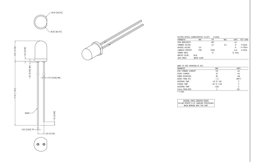
\*UNLESS OTHERWISE SPECIFIED TOLERANCES PER DECIMAL PRECISION ARE: X=±1 (±0.039), X.X=±0.5 (±0.020), X.X=±0.25 (±0.010), X.XX=±0.127 (±0.005). LEAD SIZE=±0.05 (±0.002), LEAD LENGTH=±0.75 (±0.030). MIN=  $\frac{+DECIMAL}{-DCCMAL}$  PRECISION MAX.=  $\frac{+0.00}{-DCCMAL}$
