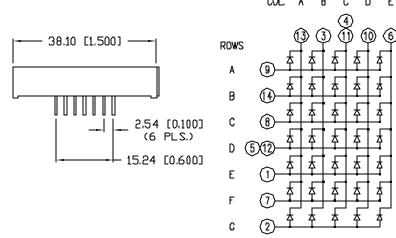
\*UNIESS OTHERWISE SPECFED TOLERANCES PER DECIMAL PRECISION ARE: X=±1 (±0.039), XX=±0.5 (±0.020), XXX=±0.25 (±0.010), XXXX=±0.127 (±0.005). LEAD 97ZE=±0.05 (±0.002), LEAD LENGTH=±0.75 (±0.030). NN= +0ECIMAL PRECISION MAX.= +0.00 (±0.000), XXXX=±0.127 (±0.005).
