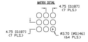
\*UNLESS DTHERWISE SPECIFIED TOLERANCES PER DECINAL PRECISION ARE: X=±1 (±0.039), X.X=±0.5 (±0.020), XXX=±0.25 (±0.010), XXXX=±0.127 (±0.005). LEAD SIZE=±0.05 (±0.002),
