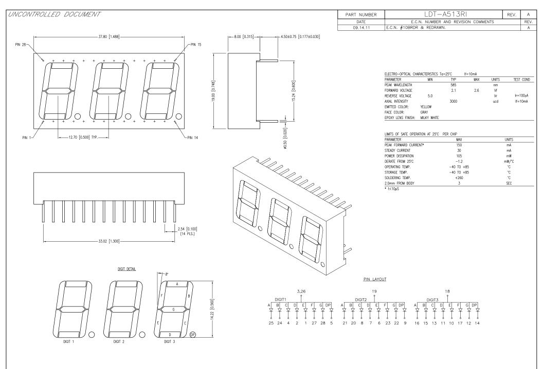
\*UNLESS OTHERWISE SPECIFIED TOLERANCES PER DECIMAL PRECISION ARE:  $x=\pm 1$  (±0.039),  $X.X=\pm 0.5$  (±0.020),  $X.XX=\pm 0.25$  (±0.010),  $X.XX=\pm 0.127$  (±0.005). LEAD SIZE=±0.05 (±0.002), LEAD LENGTH=±0.75 (±0.030). MIN=  $^{+0.001}_{-0.000}$  MAX.=  $^{+0.001}_{-0.000}$  M
