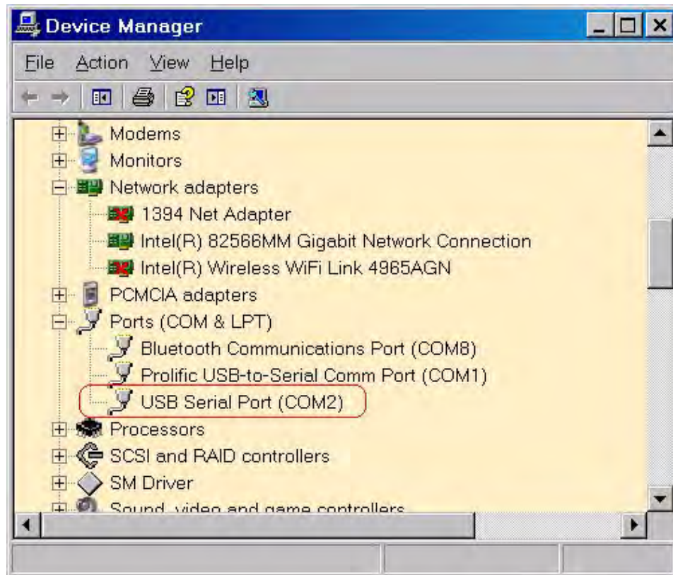
Figure 11. A Successful USB-to-UART Driver Installation
