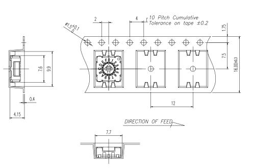
The tape and reel is applicable for Actuator 1 or 3 with Termination S or J 800 pcs/reel
