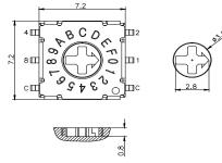
1 Slotted Spindle (Height = 3 mm)
