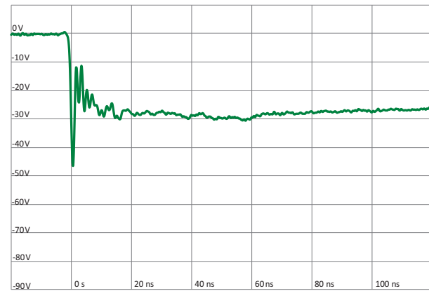
IEC 61000-4-2 -8 kV Contact ESD Clamping Voltage
