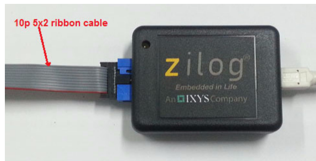
Figure 3. Connecting the 10-pin Ribbon Cable to the S3 Flash ISP II
