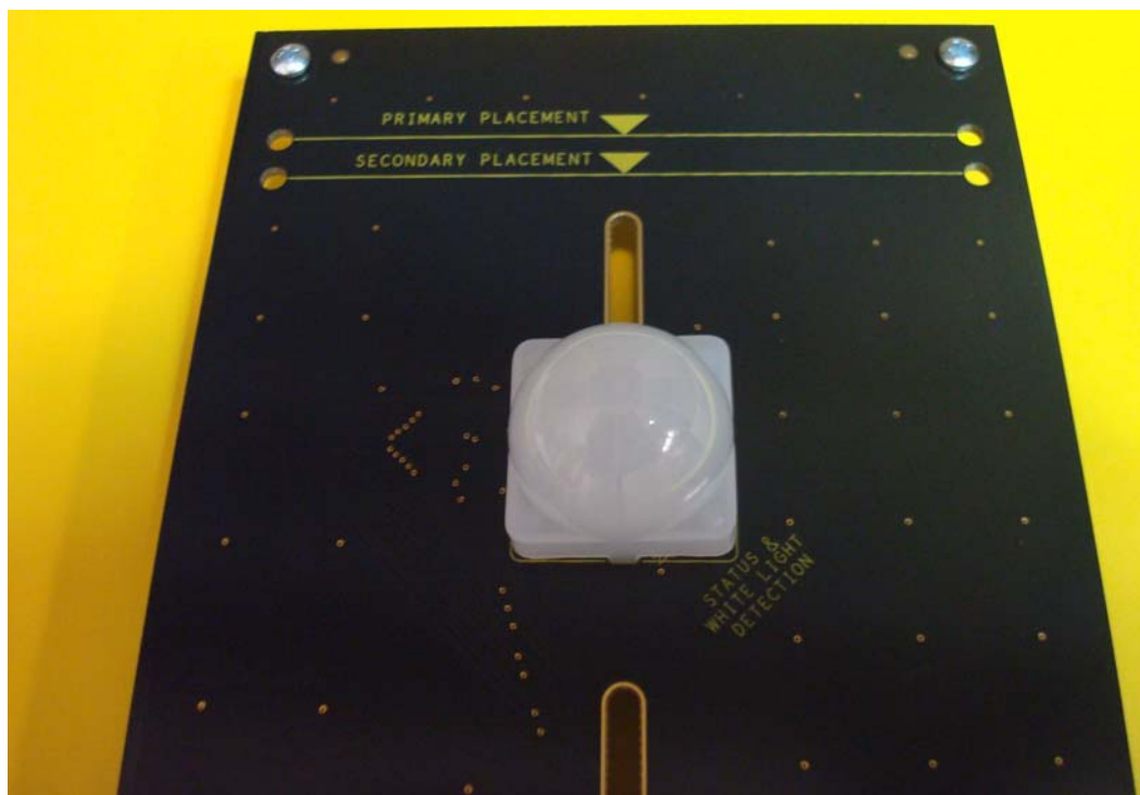
Figure 4. Assembled Clip-In Lens Installed on the ZMOTION 20-Pin Development Board
