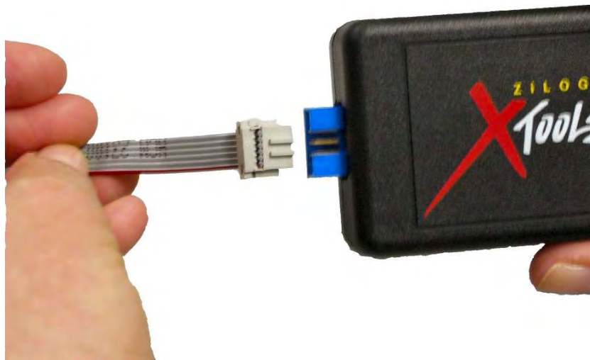
Figure 11. Connecting the Six-Conductor Ribbon Cable to the USB SmartCable
