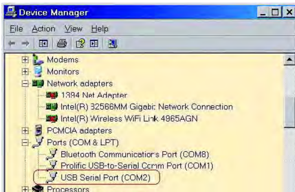
Figure 17. A Successful USB-to-UART Driver Installation
