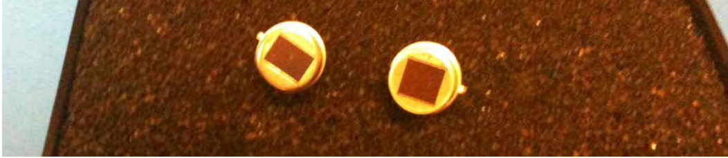
Figure 2. Two Additional Pyroelectric Sensors (L–R): SDA02-54-P and SBDI46-504AA
