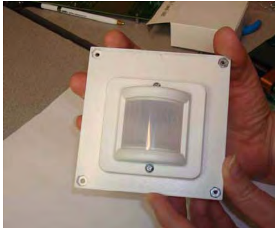
Figure 10. Assembled Flat 0.9" Lens Holder and Flat Lens
