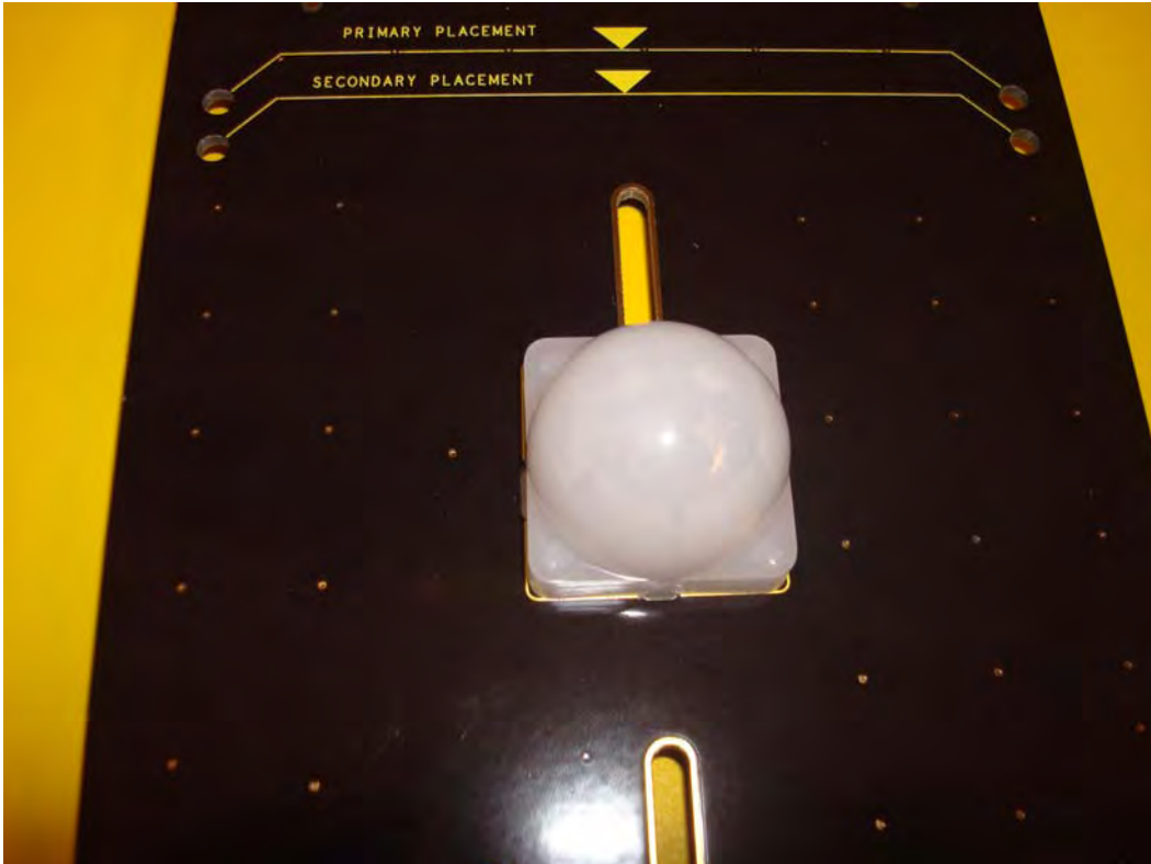
Figure 4. Assembled Clip-In Lens Installed on the ZMOTION Development Board
