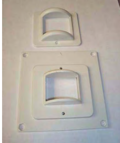
Figure 8. Flat 0.9" Lens Holder (Cap and Base)
