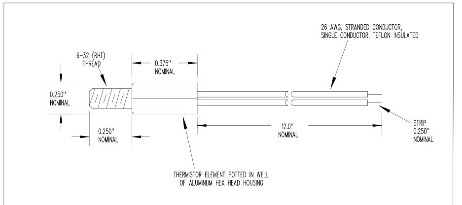
RESISTANCE @  $+25^{\circ}C = 1,000 \Omega \pm 5\%$ RESISTANCE/TEMPERATURE CURVE = "F" BETA " $\beta$ " (0 TO  $+50^{\circ}C$ ) = 3,419 K NOMINAL TEMPERATURE COEFFICIENT @  $+25^{\circ}C = -3.86\%$ /C NOMINAL TEMPERATURE RATING = -55 TO  $+150^{\circ}C$
