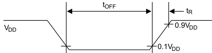
Figure 125. Low Voltage Reset Timing
