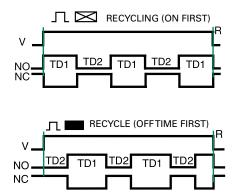
V = Voltage NO = Normally Open Contact NC = Normally Closed Contact TD1, TD2 = Time Delay R = Reset
