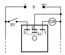
V = VoltageS1 = Initiate Switch CR = Compressor or Control Relay
