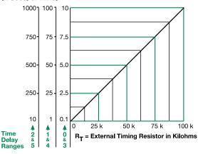
This chart applies to externally adjustable part numbers. The time delay is adjustable over the time delay range selected by varying the resistance across the  $R_T$  terminals; as the resistance increases the tie delay increases
