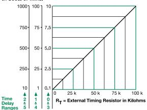
This chart applies to externally adjustable part numbers. The time delay is adjustable over the time delay range selected by varying the resistance across the  $\mathsf{R}_\mathsf{T}$  terminals; as the resistance increases the tie delay increases.
