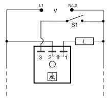
V = Voltage S1 = Optional Low Current Initiate Switch L = Load
