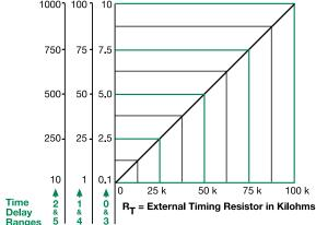
This chart applies to externally adjustable part numbers. The time delay is adjustable over the time delay range selected by varying the resistance across the  $R_T$  terminals; as the resistance increases the tie delay increases.
