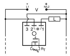
V = Voltage L = Load  $R_T$  is used when external adjustment is ordered.
