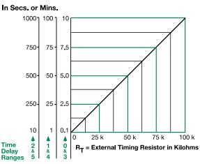
This chart applies to externally adjustable part numbers. The time delay is adjustable over the time delay range selected by varying the resistance across the  $R_T$  terminals; as the resistance increases the tie delay increases
