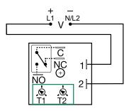
V = Voltage C = Common NO = Normally Open NC = Normally Closed T1 = OFF Time T2 = ON Time
