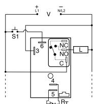
NO = Normally Open S1 = Initiate Switch L = Load C = Common, Transfer Contact
