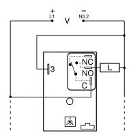
NO = Normally Open L = Load C = Common, Transfer Contact
