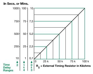
This chart applies to externally adjustable part numbers. The time delay is adjustable over the time delay range selected by varying the resistance across the RT terminals; as the resistance increases the time delay increases. When selecting an external R $_{\text{T}}$ , add the tolerances of the timer and the R $_{\text{T}}$
