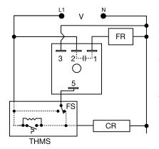
V = Voltage FR = Fan Relay FS = Fan Switch CR = Compressor Relay THMS = WallThermostat
