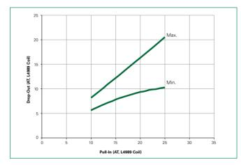
**Note:** Chart represents the range of Drop-Out, min to max, for a given Pull-in value of the MDSR-10 prior to modification into the MDSM-10.
