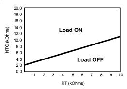
Note: If  $R_{\text{\tiny T}}$  value exceeds 13kOhms, the output will not energize.
