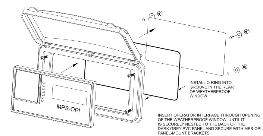
INSTALL O-RING INTO THE GROOVE IN THE REAR OF WEATHERPROOF WINDOW ASSEMBLY.
