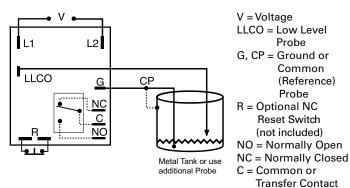
Relay contacts are isolated. Connect common to conductive tank. Additional probe is necessary for non-conductive or insulated tanks.
