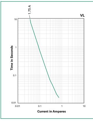
The average time current curves and Temperature Rerating curve performance is affected by a number or variables, and these curves provided as guidance only. Customer must verify the performance in their application.
