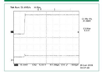
Channel 1: current through LEDs (318 mA)
