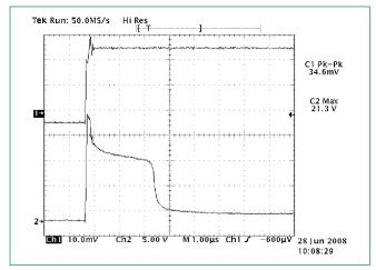
Channel 1: current through LEDs (346 mA) and PLED component once it is fully turned on 2.5 µsec later Channel 2: voltage across PLED component (21.3 V before PLED crowbars with 2 V drop)
