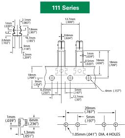
PCB MOUNTING HOLE SPECIFICATION
