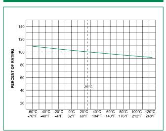
$\ensuremath{\textbf{NOTE}}\xspace$ : Derating depicted in this curve is in addition to the standard derating of 25% for continuous operation.
