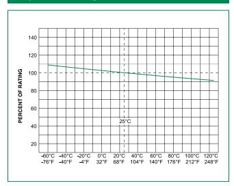
**NOTE**: Derating depicted in this curve is in addition to the standard derating of 25% for continuous operation.
