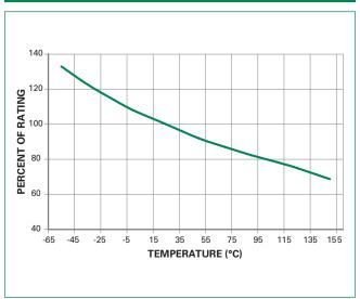
1. Rerating depicted in this curve is in addition to the standard derating of 20% for continuous operation.
