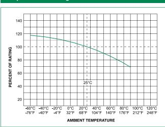
**Notes:** Rerating depicted in this curve is in addition to the standard derating of 25% for continuous operation. Example:
