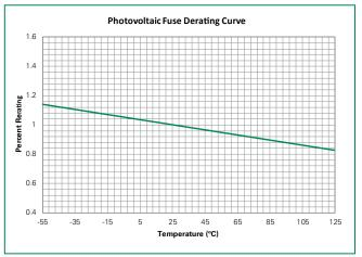
$\ensuremath{\textbf{Note:}}$  Rerating depicted in this curve is in addition to the standard derating of 25% for continuous operation.
