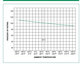
Note: Rerating depicted in this curve is in addition to the standard derating of 25% for continuous operation.
