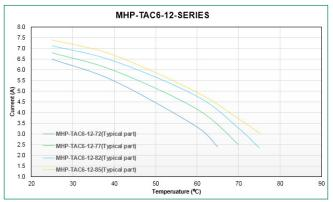
The current vs. temperature curve was derived from placing test samples in an oven at 25°C, 40°C, 60°C, 70°C, 75°C, and 80°C, increasing current flow through the sample at a rate of 0.1 A/minute and recording the current value when the sample trips.
