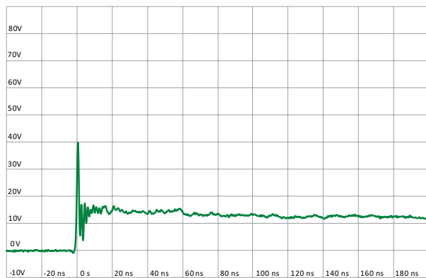
IEC 61000-4-2 +8 kV Contact ESD Clamping Voltage
