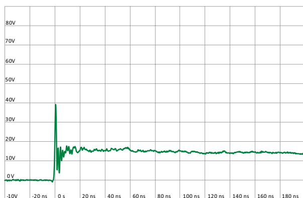
ISO10605 Contact Discharge Plot at +8 kV
