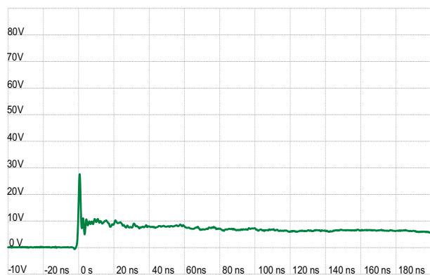
ISO10605 Contact Discharge Plot at +8 kV
