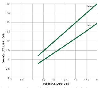
${\tt Note: Chart\ represents\ the\ range\ of\ Drop-Out,\ min\ to\ max\ for\ a\ given\ Pull-In\ value.}$
