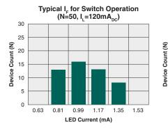
Typical I<sub>F</sub> for Switch Dropout (N=50, I<sub>L</sub>=120mA<sub>DC</sub>)
