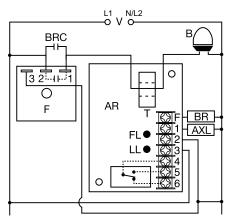
V = Voltage B = Beacon F = Flasher T =Toroid BRC = Flasher Bypass Relay Contacts AR = FB Alarm Relay BR = Bypass Relay Coil FL = Flasher Failure LED LL = Lamp Failure LED AXL = Lamp Alarm Relay Coil
