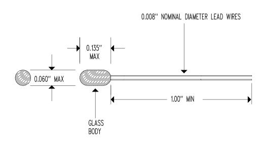
RESISTANCE @  $+25^{\circ}$ C = 10,000  $\Omega$  ± 1% RESISTANCE/TEMPERATURE CURVE = "J" BETA " $\beta$ " (+25 TO +85°C) = 3,977′K NOMINAL DISSIPATION CONSTANT = 0.75 mW/°C NOMINAL (STILL AIR) THERMAL TIME CONSTANT = 0.35 SECONDS NOMINAL (STIRRED OIL) MAXIMUM TEMPERATURE RATING =  $+300^{\circ}$ C
