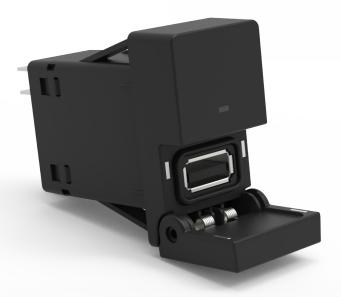
The USB CV-Charger is designed to charge electronic devices compatible with 2.0 or 3.1 USB types. The CV-Charger delivers fast charging times even in extreme temperatures from -40 °C to +85 °C. This innovative product features a spring-loaded access door that automatically closes to safeguard its electronics, assuring prolonged safe and reliable operation. The center LED indicates charging is in progress.
