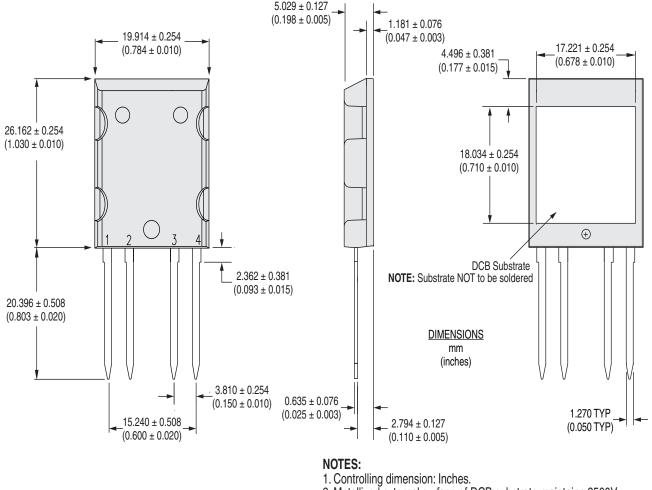
Metallized external surface of DCB substrate maintains 2500V<sub>rms</sub> isolation to device internal structure and all external pins.
