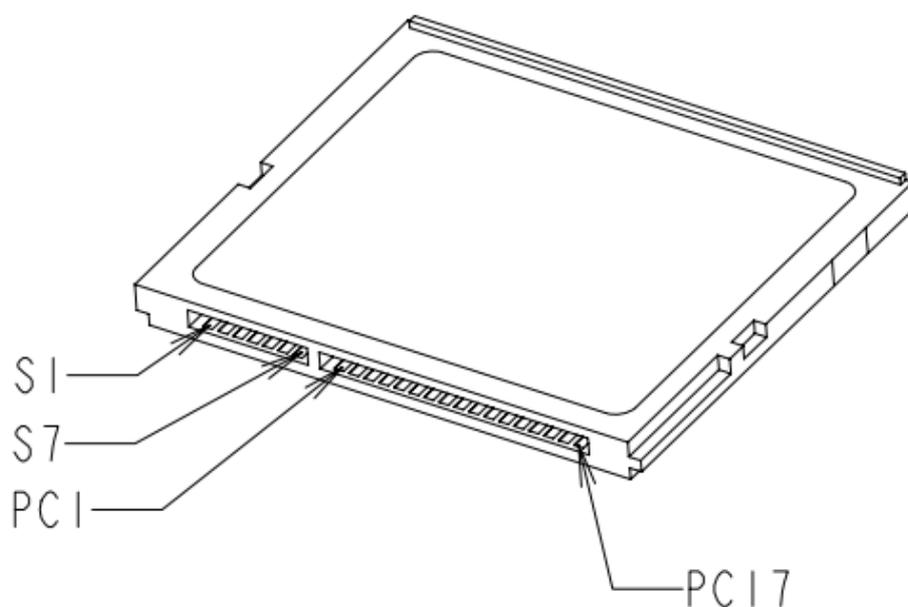
Figure 3-1 Pin Assignment
