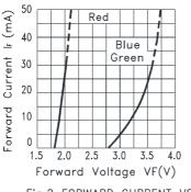
Fig.2 FORWARD CURRENT VS. FORWARD VOLTAGE
