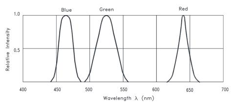
Fig.1 RELATIVE INTENSITY VS. WAVELENGTH
