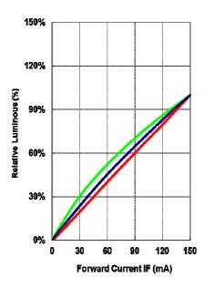
Fig 4. Forward Current vs. Relative Luminous Flux
