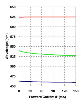
Fig 6. Forward Current vs. Dominant Wavelength
