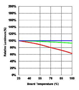
Fig 5. Board Temperature vs. Relative Luminous Flux *Note:*
