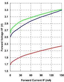
Fig 3. Forward Current vs. Voltage
